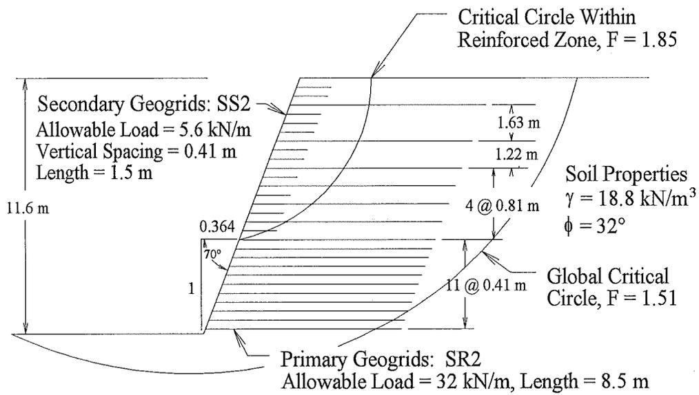
Figure 1: 70 Degree Slope Designed Using Tensar Guidelines, Showing Internal and External Critical Circles.
