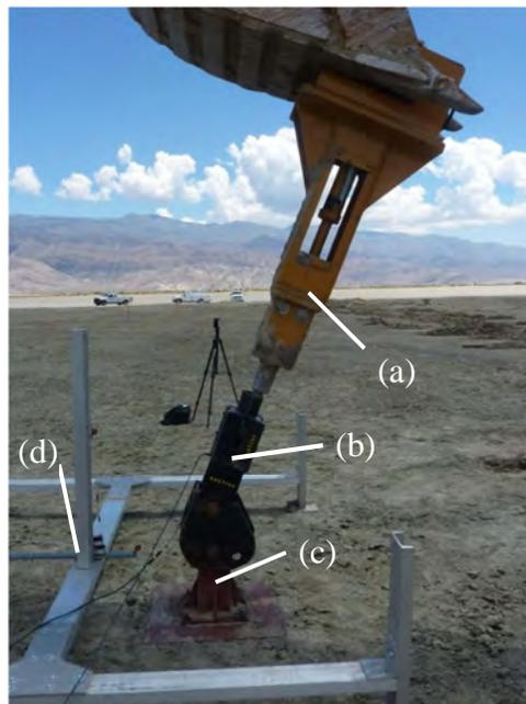
**Figure 3. Test system showing (a) excavator attachment, (b) Instrumented swivel unit, (c) foundation attachment, (d) reference frame with position sensors**
