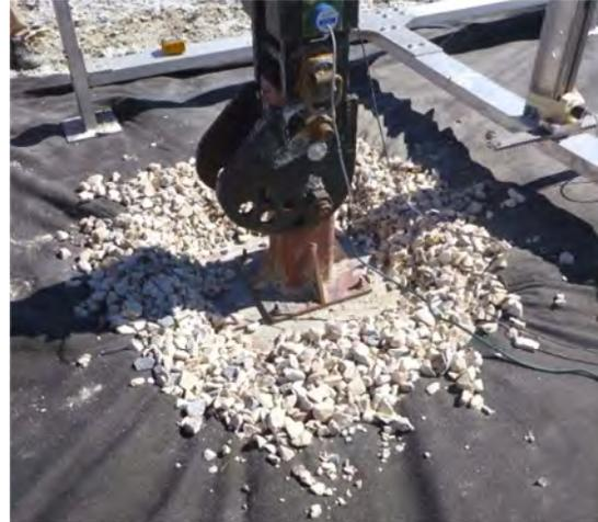
**Figure 11. Footing test with fabric and gravel after a plate test**
