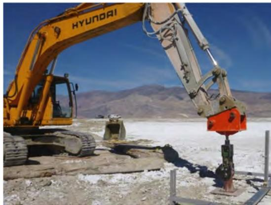
Figure 4. Direct push attachment with pin grabber
