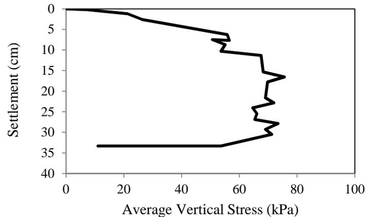
**Figure 12. Typical settlement versus pressure graph with bearing failure
