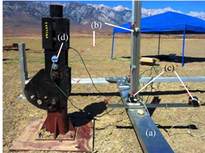
**Figure 9. Measurement system showing (a) reference, (b) tether lines and pulleys, (c) potentiometers, and (d) tiltmeter**
