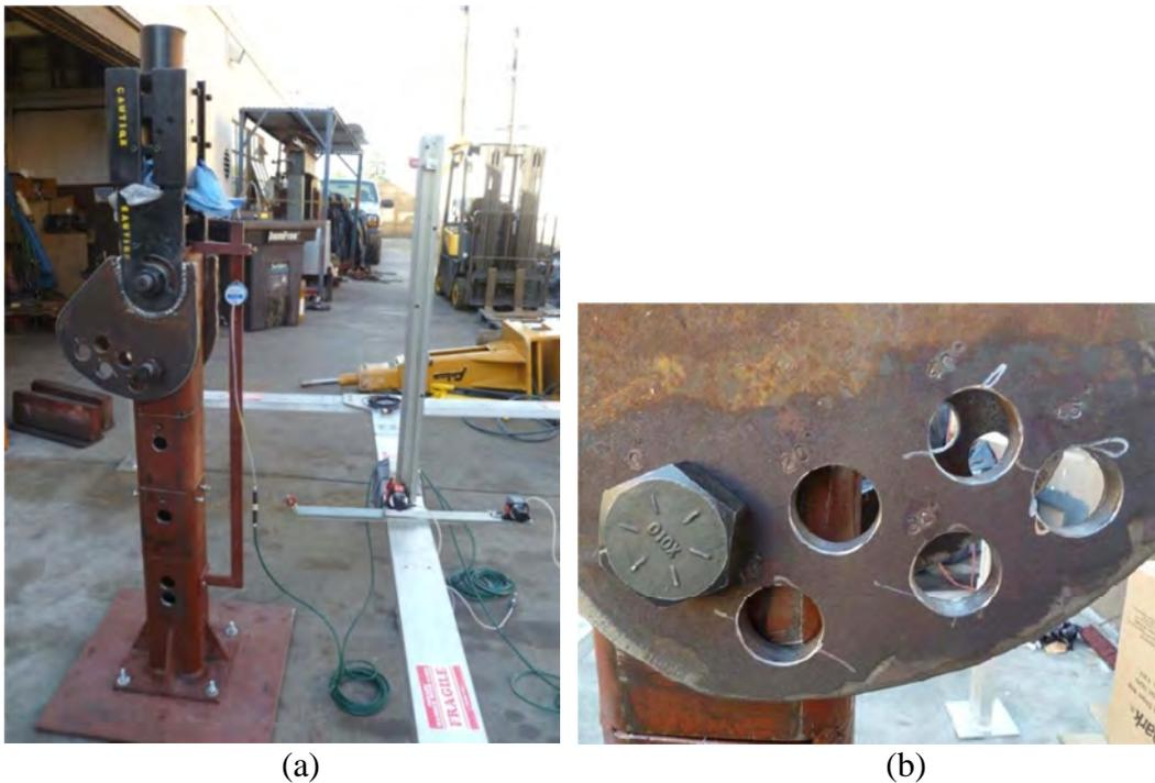
Figure 7. (a) Swivel unit bolted on the footing stem and (b) detail of preset positions to set the swivel unit angle to 0°, 10°, 20°, 30°, 40°, or 45°
