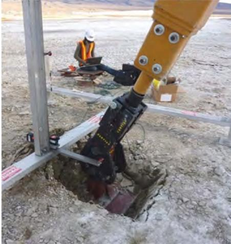
**Figure 10. Footing test after applying an inclined load**
