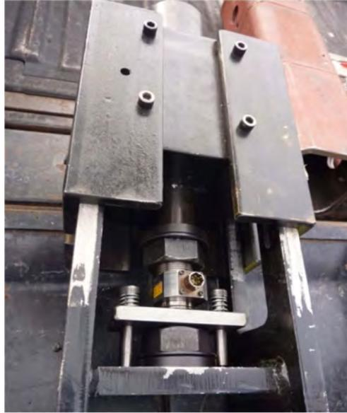
Figure 6. Load cell held inside the swivel unit
